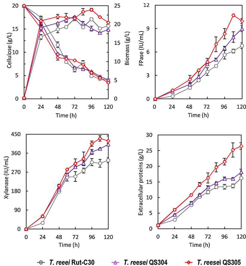
Fig. 5. Cellulase production by *T. reesei* QS304, QS305 and Rut-C30 under submerged culture conditions in the 5-L fermentor. Averages of the duplicate are shown with standard deviations.
